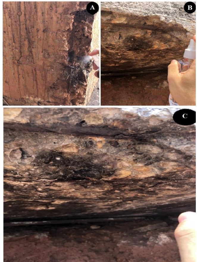
Fig. 7. A) Carbonation test on the pillar; B and C) Carbonation test on the tray
