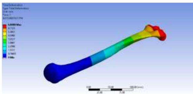
Fig. 3: Shows the Maximum total Deformity in Normal bone
