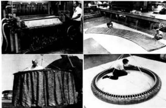
Fig. 3: Manufacturing of Nozzle Extension, taken from [9]
