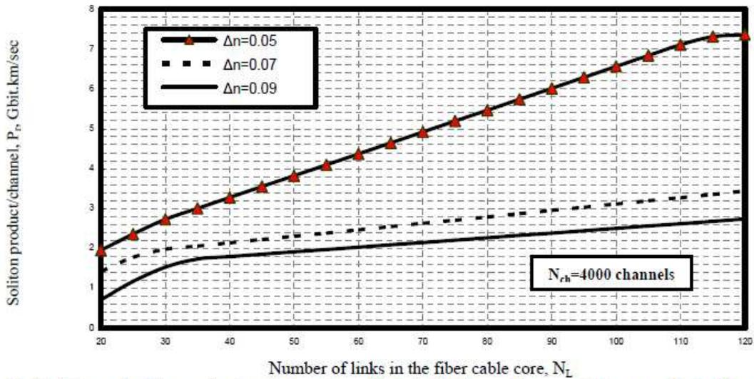
Fig. 10. Variations of soliton product against number of links in the fiber cable core at the assumed set of parameters.
