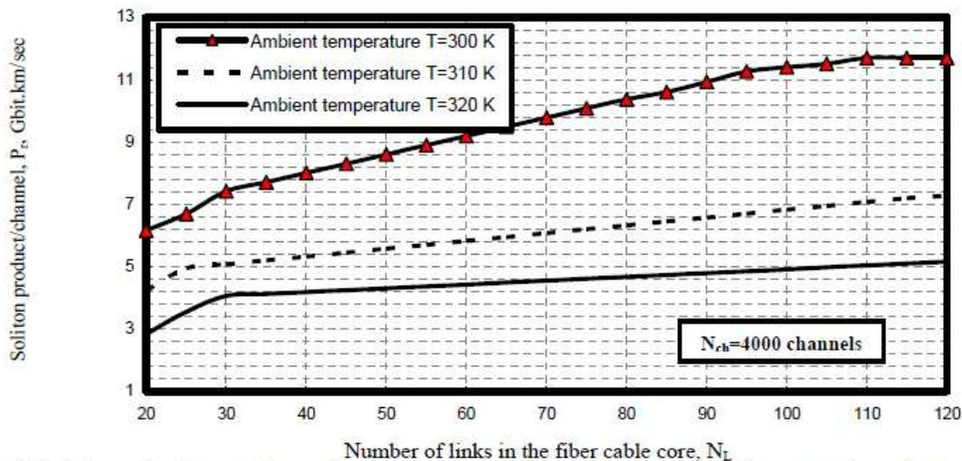
Fig. 6. Variations of soliton product against number of links in the fiber cable core at the assumed set of parameters.
