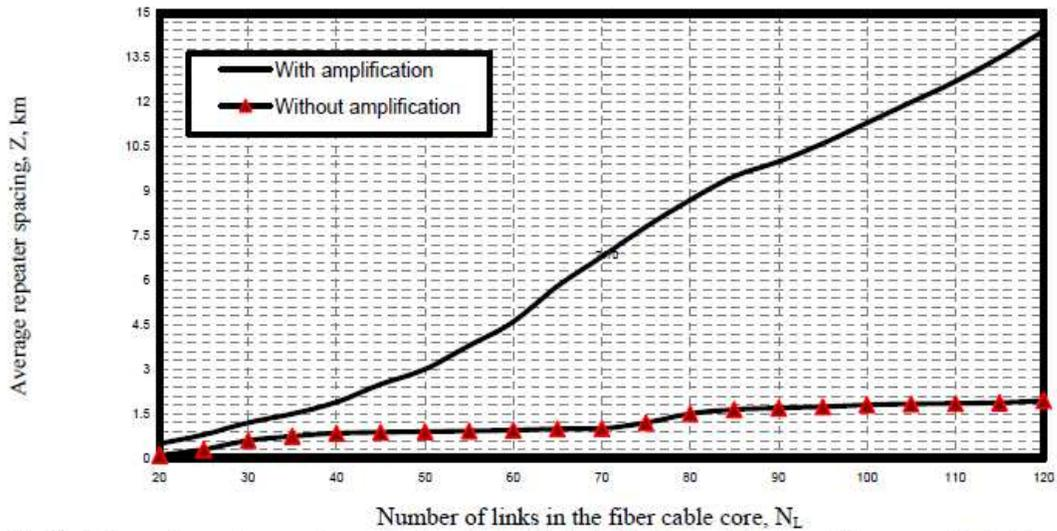
Fig. 11. Variations of repeater spacing against number of links in the fiber cable core at the assumed set of parameters.
