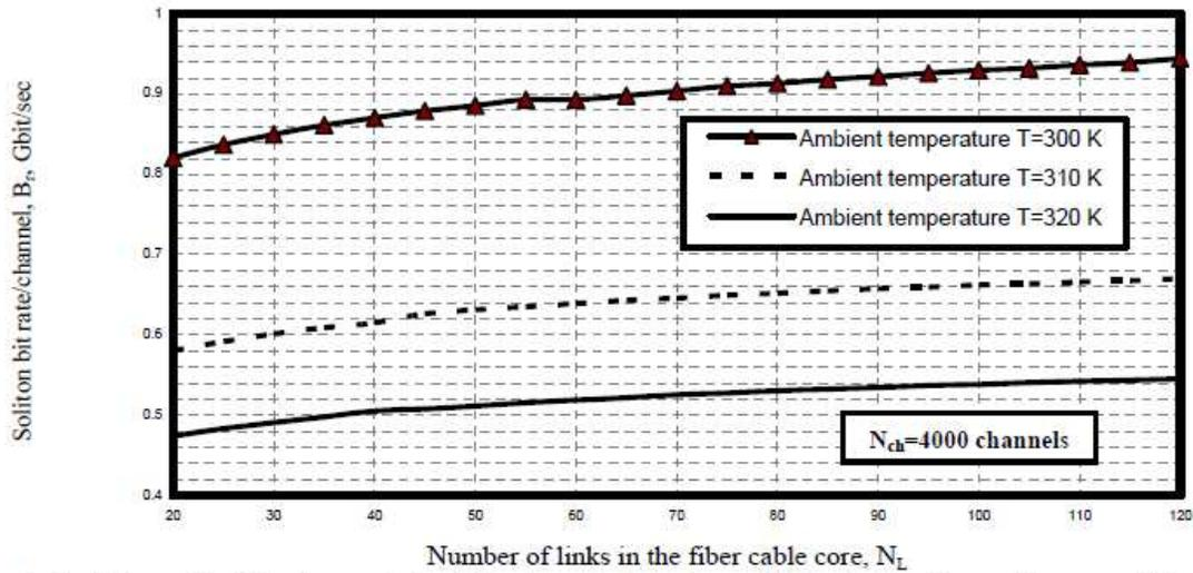
Fig. 4. Variations of soliton transmission bit rate against number of links in the fiber cable core at the assumed set of parameters.
