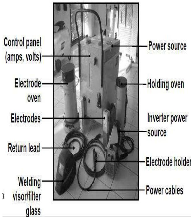
Fig.1 (b). Manual Metal Arc Welding Basic Equipment
