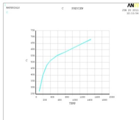
Fig.7. Thermal specific of carbon steel
