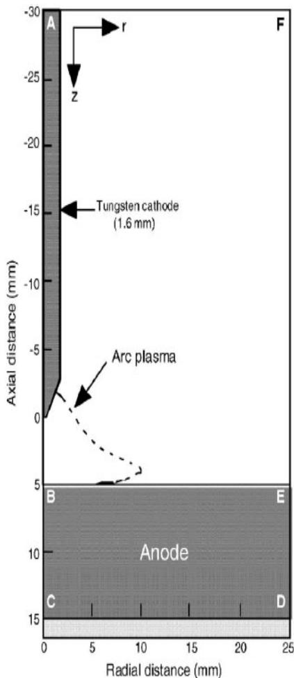
Fig. 2. Arc-electrode model [8]
