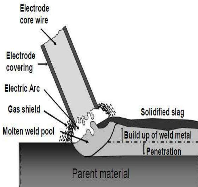
Fig. 1 (a). Manual Metal Arc Welding (MMAW) Process
