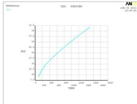
Fig.6. Thermal conductivity of carbon steel
