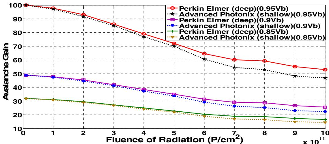
Fig. 2. Variations of avalanche gain against fluence of radiation at the assumed set of parameters.
