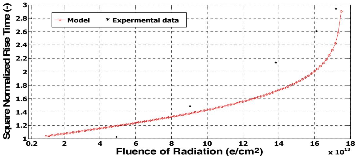
Fig. 8. Variations of the square normalized rise time against fluence of radiation at the assumed set of parameters.
