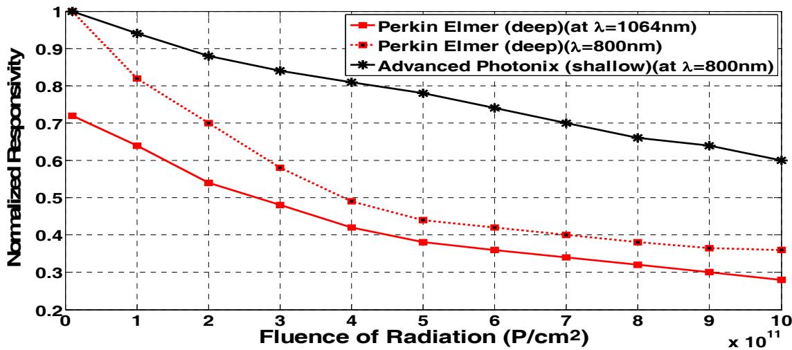
Fig. 7. Variations of the normalized responsivity against fluence of radiation at the assumed set of parameters.
