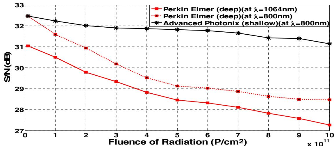
Fig. 9. Variations of the signal to noise ratio against fluence of radiation at the assumed set of parameters.
