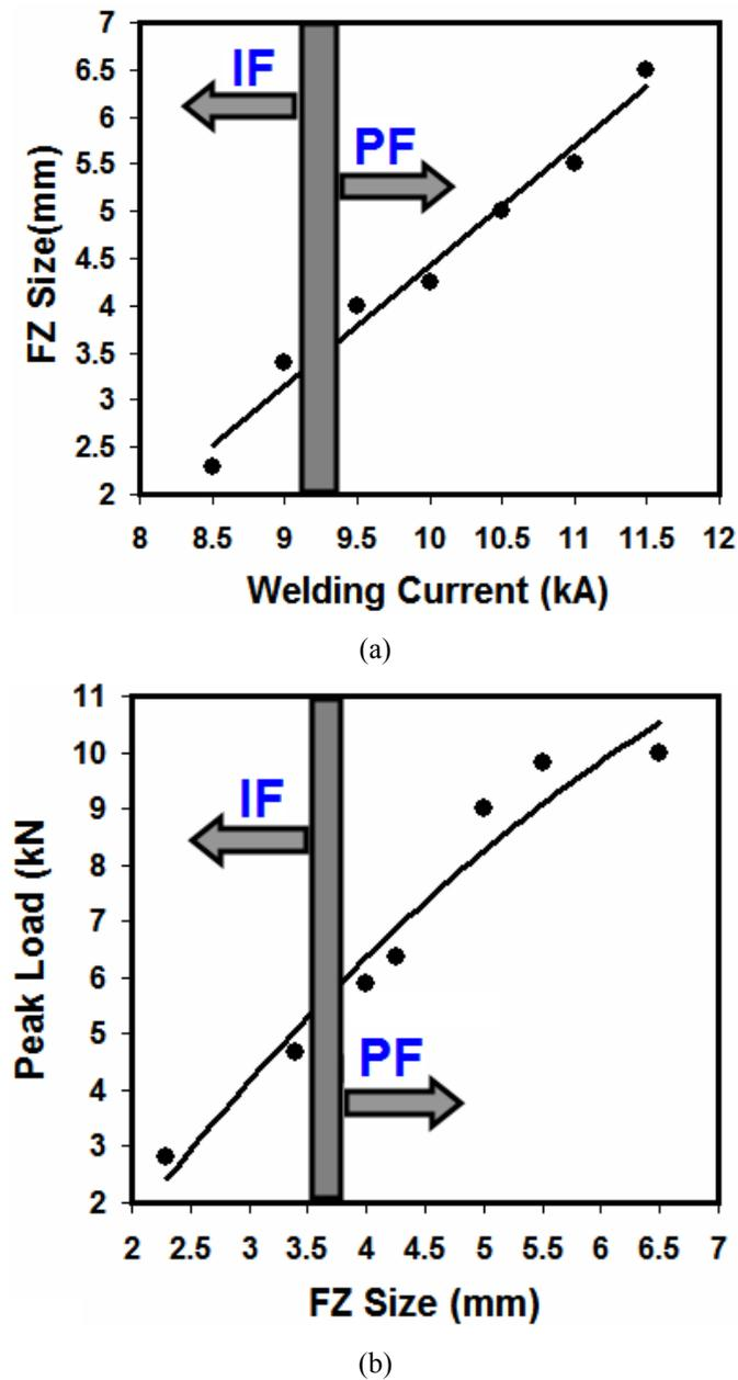
Fig. 6. (a) Effect of welding current on FZ size, (b) effect of FZ size on the peak load
