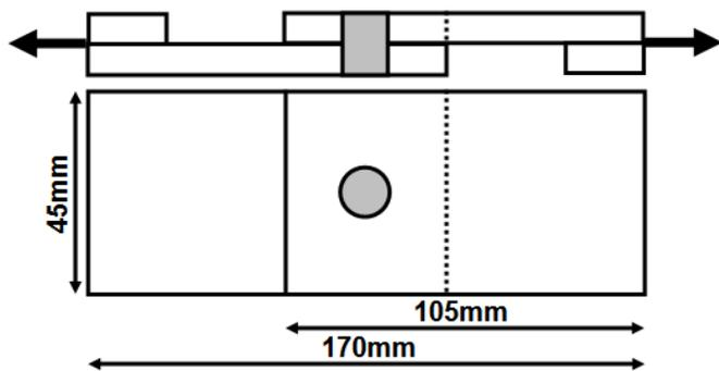
Fig. 2. Sample dimensions for tensile-shear test
