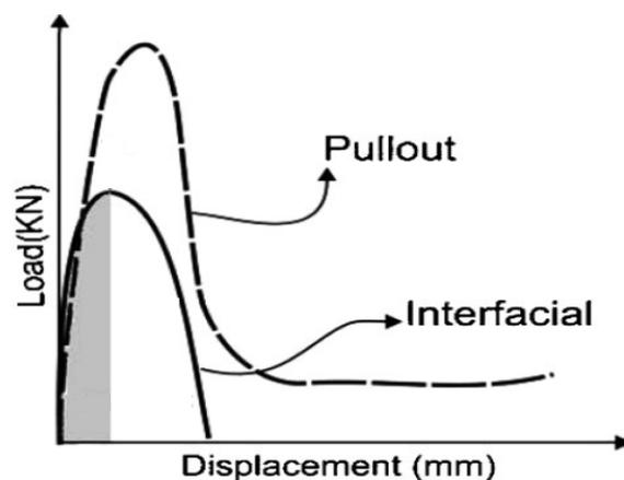
Fig. 1. Load displacement curve for both failure modes
