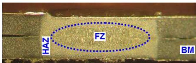
Fig. 3. A typical macrostructure of low carbon steel resistance spot weld
