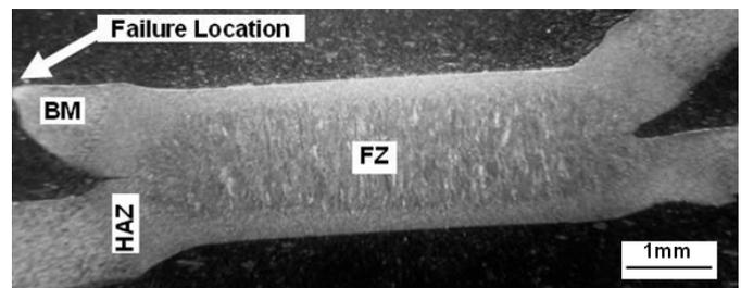
Fig. 7. Cross section of fracture surfaces of spot welds in tensile-shear test: One leg of the lower sheet and one leg of the upper are subjected to tensile stress.
