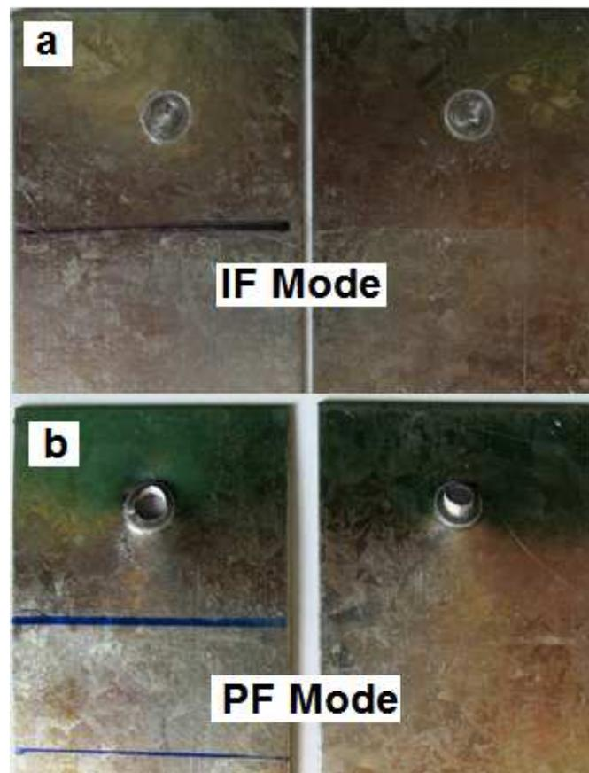
Fig. 5. Observed spot weld failure modes: (a) interfacial, (b) nugget pullout
