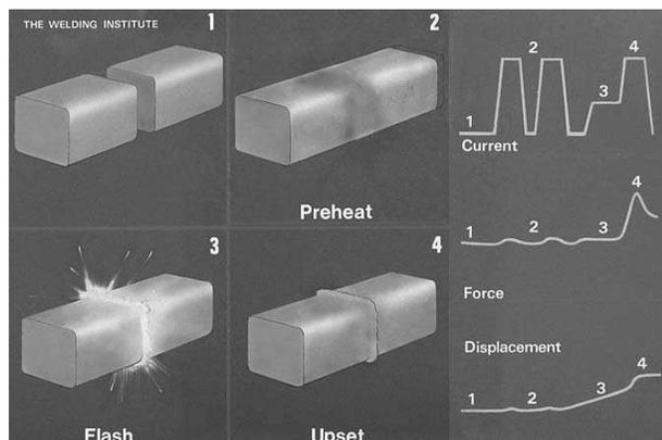
Fig. 6: Principles of flash butt welding. Courtesy of TWI Ltd
