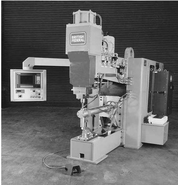
Fig. 2: Modern pedestal mounted spot welder for aerospace applications
