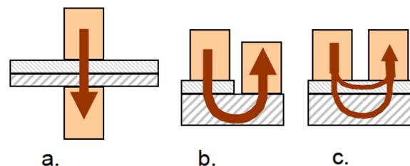
Fig. 8: Examples of resistance welding electrode configurations: a) direct, b) step, and c) series
