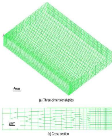
Fig. 4: Finite-Element Modeling of Resistance Welding
