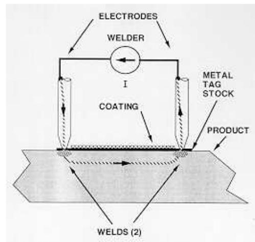
Fig.1: Principles of spot welding process
