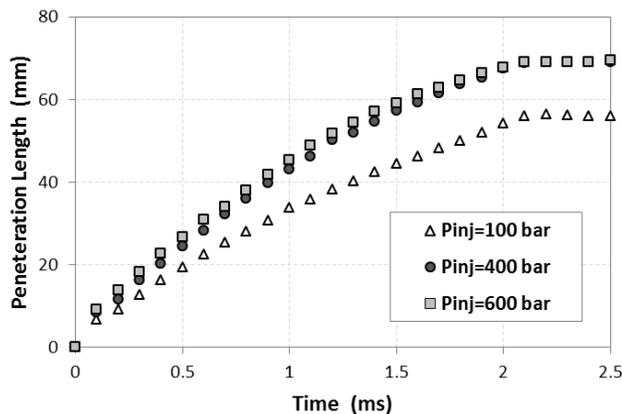
Figure 10: Spray tip penetration variation with time for different injection pressures, ( $P_{amb}=50$  bar and  $T_{amb}=683$  K)
