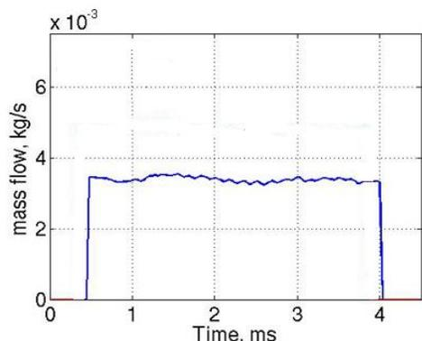
Figure 1: The injection mass flow rate profile of the single-hole injector under consideration
