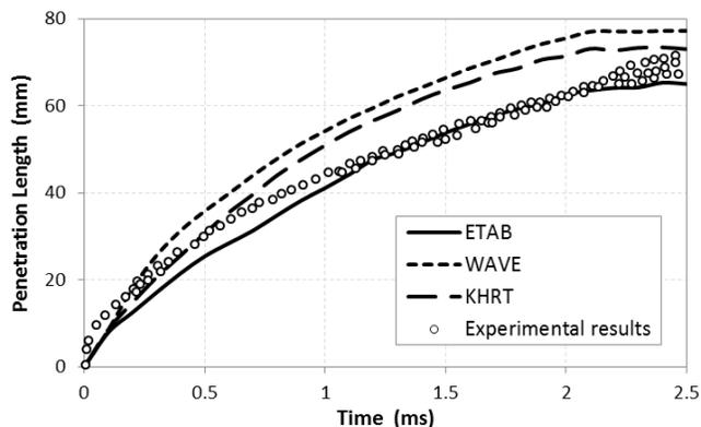
Figure 3: Comparing different breakup models abilities in predicting the spray tip penetration,  $P_{inj}=600$  bar,  $P_{amb}=50$  bar,  $T_{amb}=683$  K, spray angle=15°
