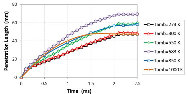
Figure 8: Spray tip penetration variation with time for different ambient temperatures, ( $P_{inj}=600$  bar and  $T_{inh}=320$  K,  $P_{amb}=50$  bar)
