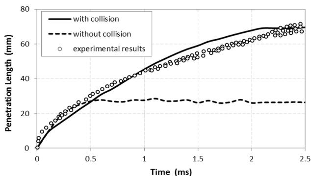
Figure 2: Effect of droplet collision modeling on spray tip penetration
