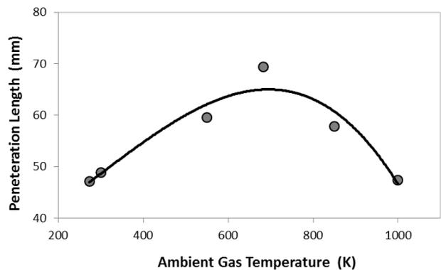
Figure 9: Spray tip penetration variation versus ambient temperature, ( $P_{inj}=600$  bar and  $T_{inh}=320$  K,  $P_{amb}=50$  bar)
