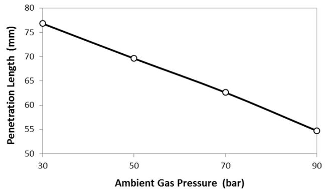
Figure 7: Spray tip penetration variation versus ambient pressure, ( $P_{inj}=600$  bar and  $T_{amb}=683$  K)
