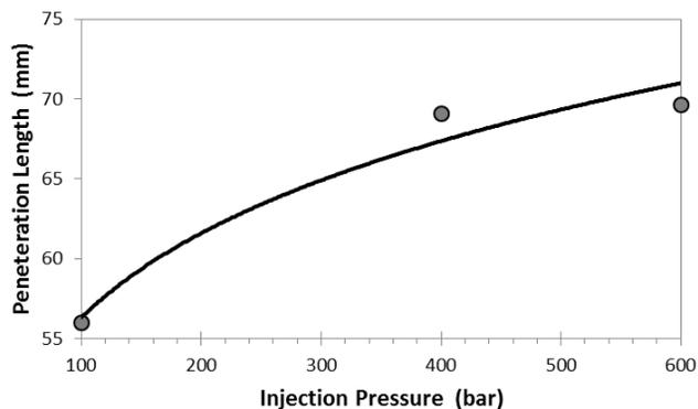
Figure 11: Spray tip penetration variation versus injection pressure, ( $P_{amb}=50$  bar and  $T_{amb}=683$  K)
