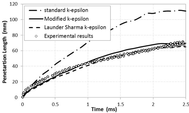
Figure 5: Comparing different turbulence models abilities in predicting the spray tip penetration, ( $P_{inj}=600$  bar,  $P_{amb}=50$  bar,  $T_{amb}=683$  K, spray angle= $15^\circ$ )
