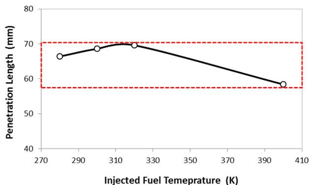
Figure 13: Spray tip penetration variation versus injection temperature
