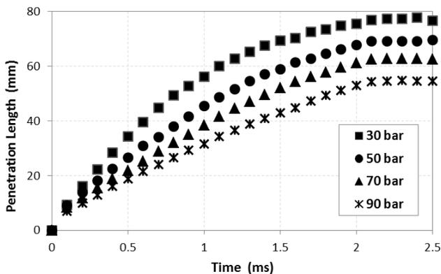
Figure 6: Spray tip penetration variation with time for different ambient pressures, ( $P_{inj}=600$  bar and  $T_{amb}=683$  K)
