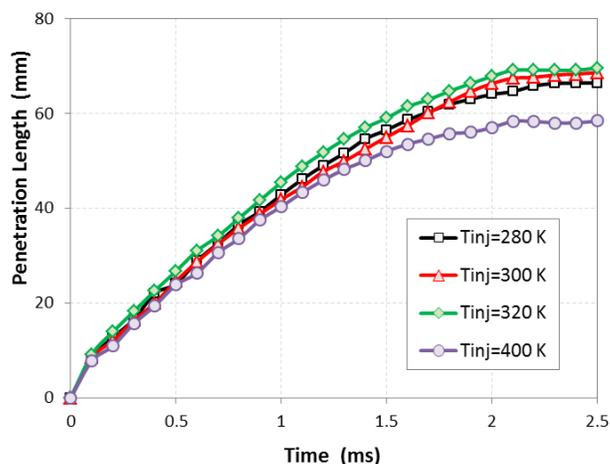
Figure 12: Spray tip penetration variation with time for different injection temperatures
