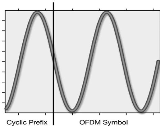
Fig. 8: Cyclic Extension of Sinusoid
