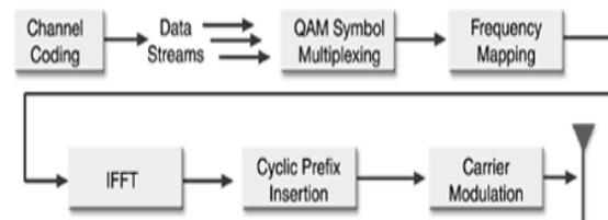
Fig. 7: OFDM transmitter chain
