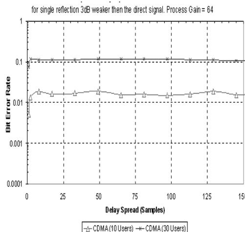
Fig. 3: Bit Error Rate Vs Multipath delay/hindrance spread for Code Division Multiple Access reverse/overturn link
