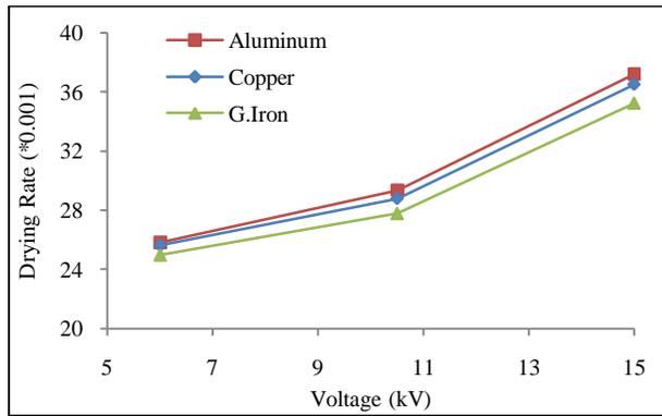
Fig. 2. Variation of drying rate with material type of grounded electrode
