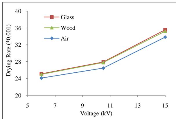
Fig. 3. Variation of drying rate with material type of box
