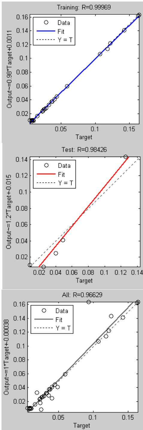
Fig. 5: Performance of training, test and all data in designed MLPNN in study 1
