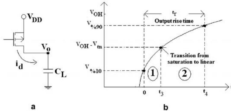
Fig. 3: (a) Load capacitance charges through PMOS transistor, (b) Output voltage waveform during low-to-high transition [17], [18]
