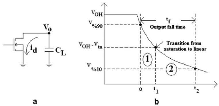
Fig. 2: (a) Load capacitance discharges through NMOS transistor, (b) Output voltage waveform during high-to-low transition [17], [18]
