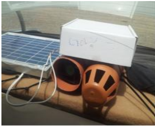
Fig. 2: Ventilation system mounted on the rear end of the car
