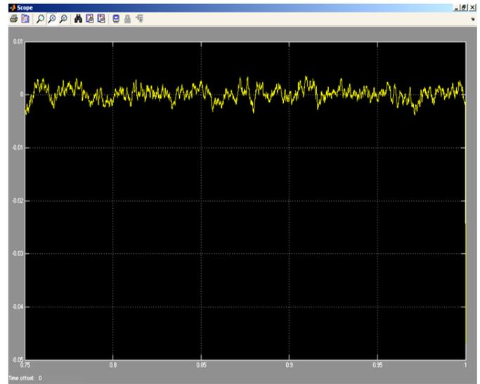
Fig. 15. Shows that the output with variable proportional controller and other two gains fixed minimized the noise.
