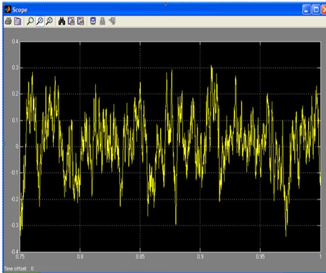
Fig. 8. Output of feed-forward compensator without compensation for  $T_F=1$ ,  $k_{ccd}=5$  and  $k_d/a=0.001$ .
