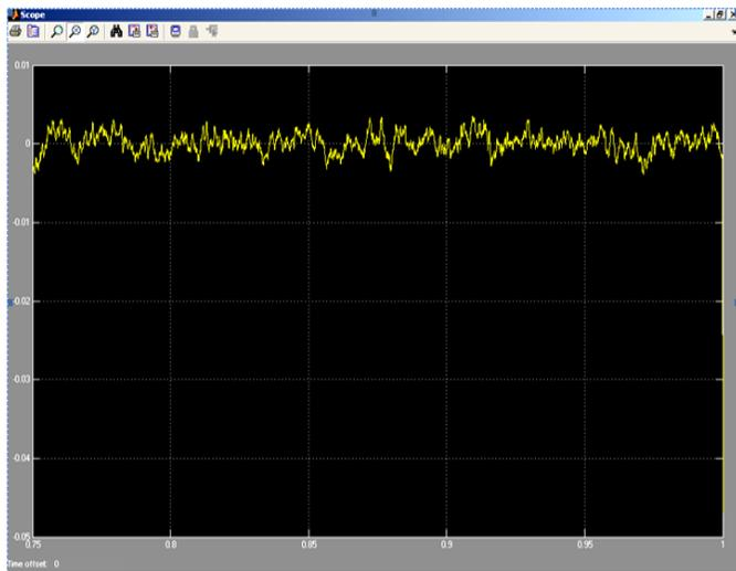
Fig. 14. Output with variable proportional controller and other two gains are fixed. (Here plant=0.33, TF2&TF1 =1, P =300, I=D=1)
