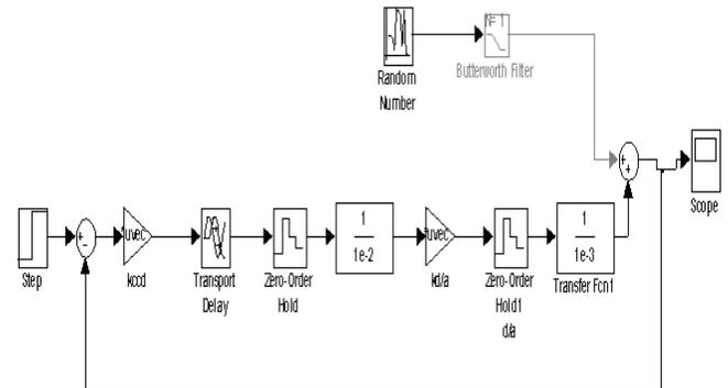
Fig. 11. Circuit diagram with variable transfer function and fixed gain
