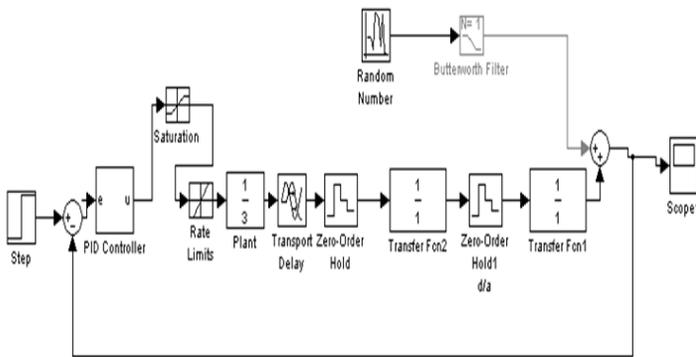
Fig. 13. Circuit diagram with variable proportional controller and other two gains fixed
