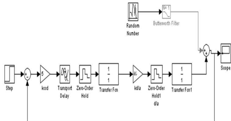
Fig. 5. Circuit diagram of Feed forward compensator without compensation
