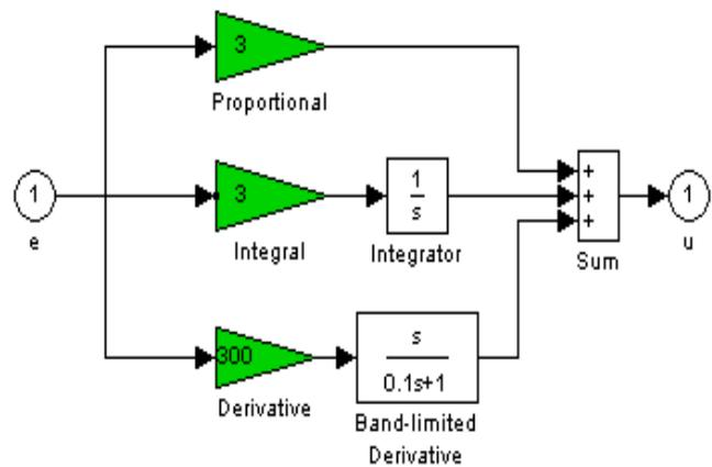
Fig. 6. Internal construction of PID block
