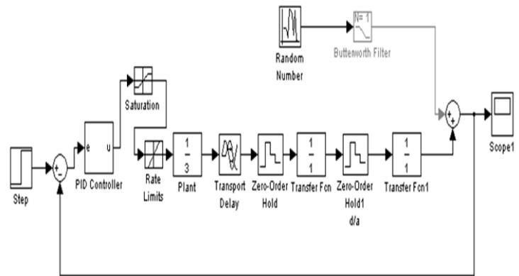
Fig. 7. Simulation diagram with PID controller
