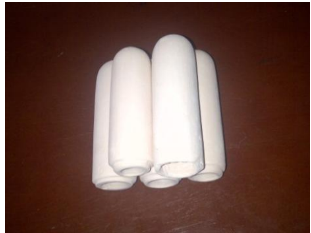
Fig. 4. Water filter candles that have been fired
