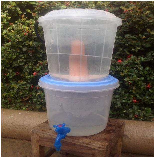
Fig. 3. The filtration set-up (1)
