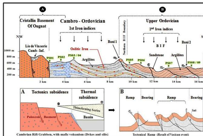
Fig. 4: Structural cross-section of the studied transects, with position sample groups (PS) (Cambrian-Ordovician series). (A) Simplified sketch of tectonic subsidence, (B) Simplified sketch of thermal subsidence in the Tafilalt basin with illustration of tectonic ramps
