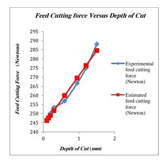
Fig. 3. Feed cutting force versus depth of cut
