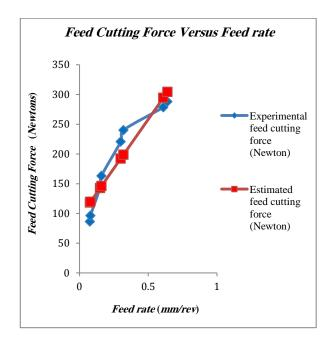
Fig. 4. Feed cutting force versus feed rate
