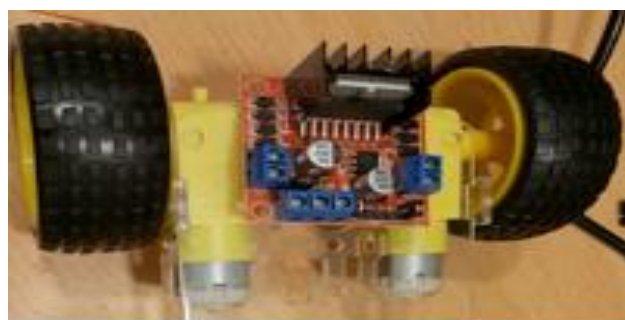
Fig. 4. The L298 Dual H-Bridge Motor Driver fixed to the body frame
