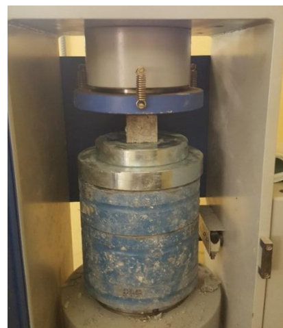
Fig. 6: Crushing of concrete cube specimen
