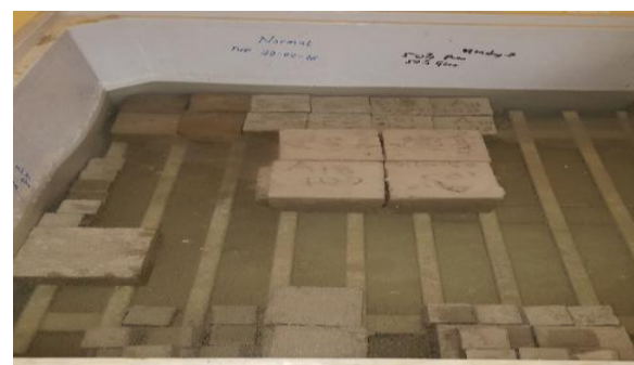
Fig. 5: Concrete specimen in Curing Tank
