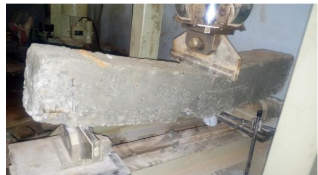
Fig. 10: Failure of beam under applied maximum load
