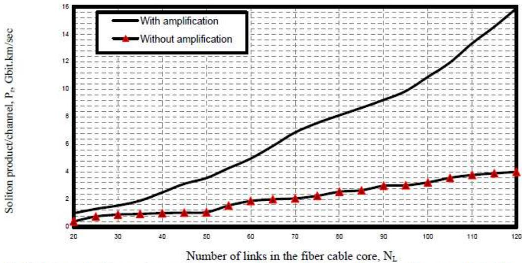
Fig. 12. Variations of soliton product against number of links in the fiber cable core at the assumed set of parameters.
