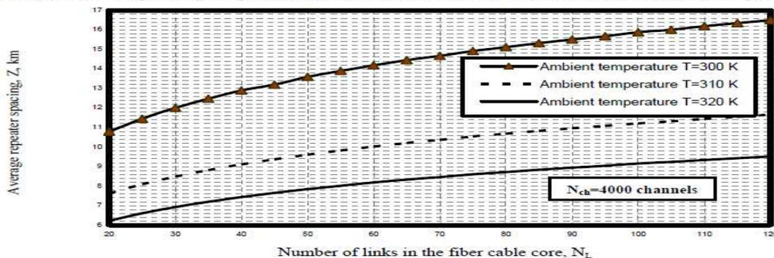
Fig. 2. Variations of repeater spacing versus number of links in the fiber cable core at the assumed set of parameters.
