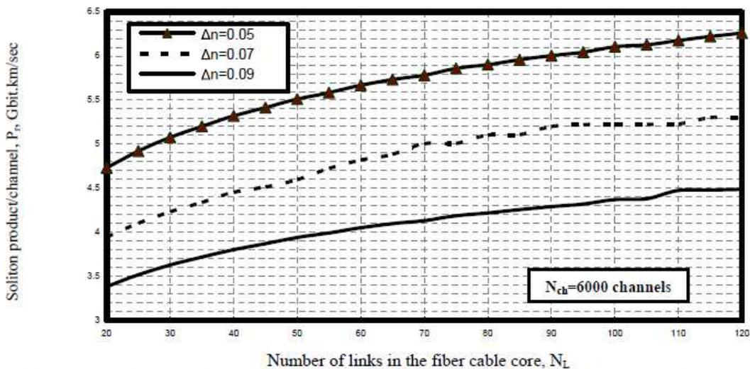
Fig. 9. Variations of soliton product against number of links in the fiber cable core at the assumed set of parameters.
