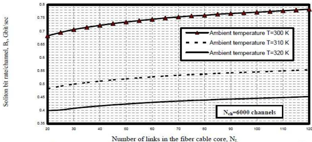
Fig. 3. Variations of soliton transmission bit rate against number of links in the fiber cable core at the assumed set of parameters.
