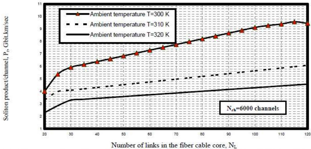
Fig. 5. Variations of soliton product against number of links in the fiber cable core at the assumed set of parameters.
