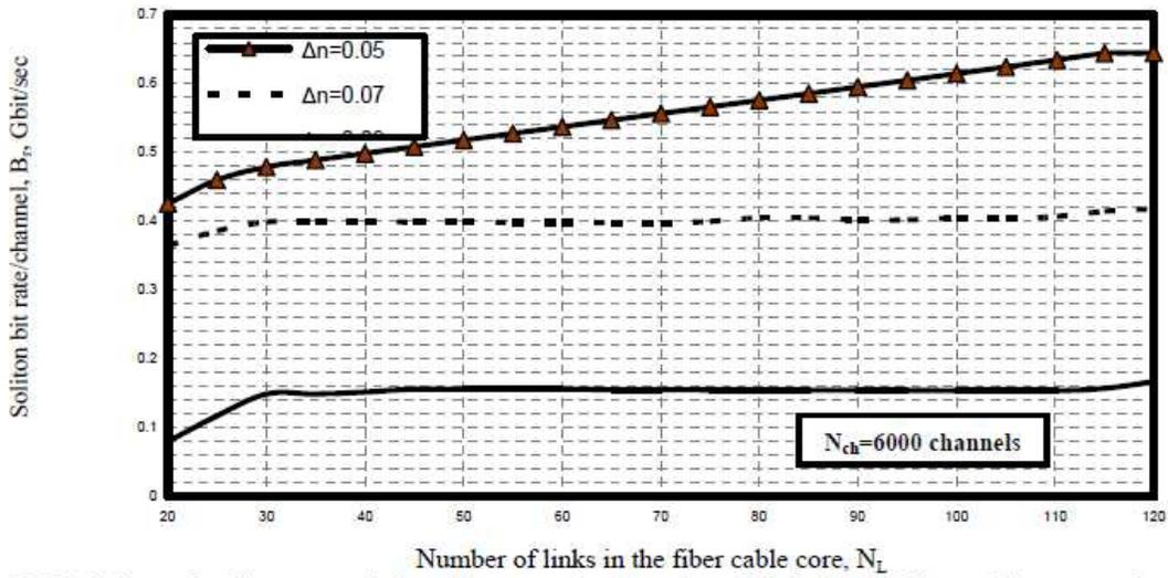
Fig. 7. Variations of soliton transmission bit rate against number of links in the fiber cable core at the assumed set of parameters.
