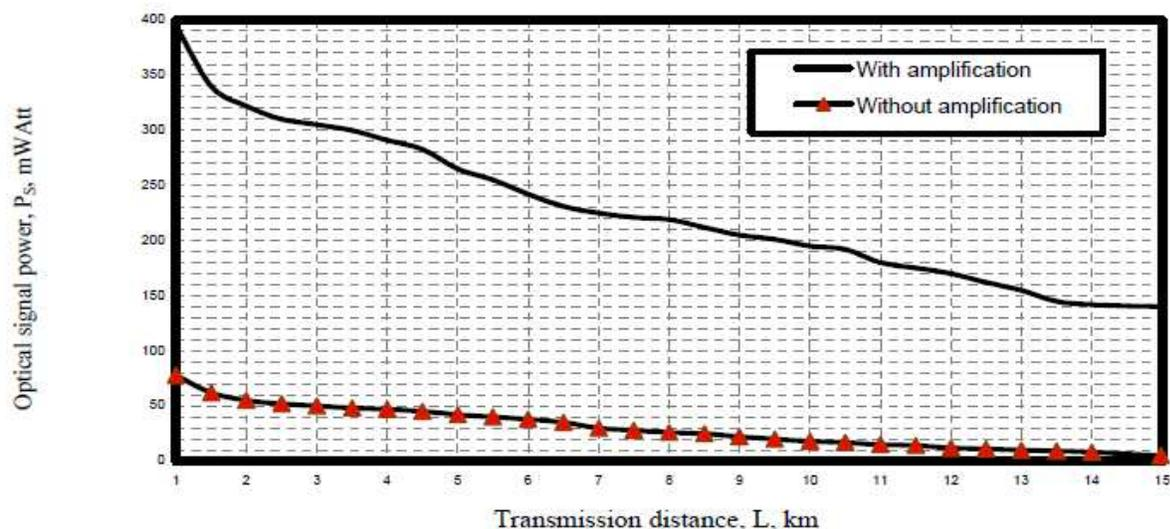
Fig. 13. Variations of optical signal power against average repeater spacing at the assumed set of parameters.
