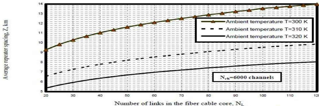
Fig. 1. Variations of repeater spacing versus number of links in the fiber cable core at the assumed set of parameters.
