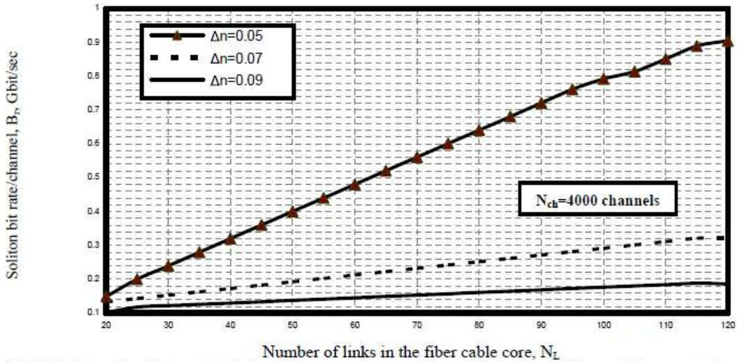
Fig. 8. Variations of soliton transmission bit rate against number of links in the fiber cable core at the assumed set of parameters.
