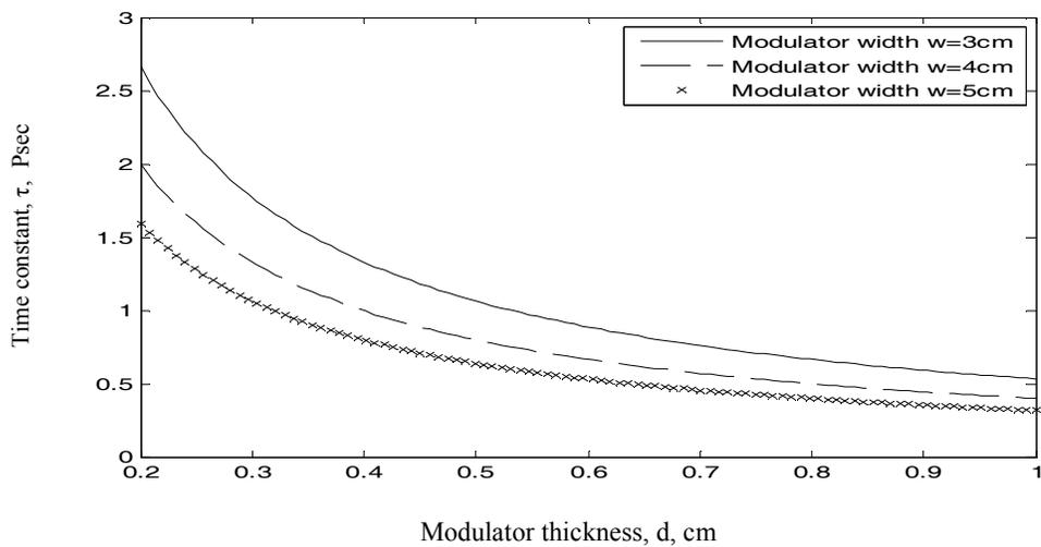
Fig. 7. Variations of modulator time constant against modulator thickness at the assumed set of parameters.
