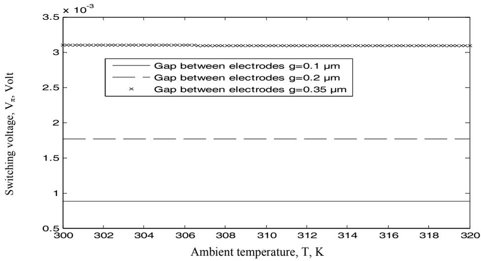
Fig. 5. Variations of the switching voltage against ambient temperature at the assumed set of parameters.
