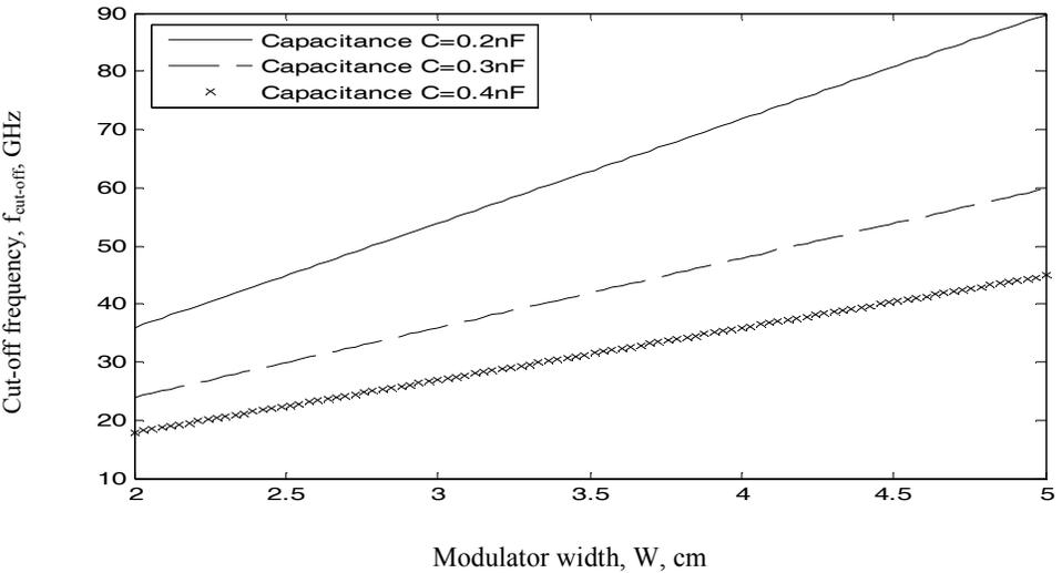
Fig. 9. Variations of cut-off frequency against modulator width at the assumed set of parameters.
