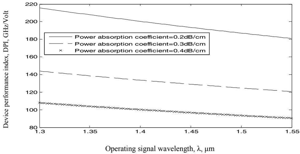
Fig. 2. Variations of the device performance index versus operating signal wavelength at the assumed set of parameters.
