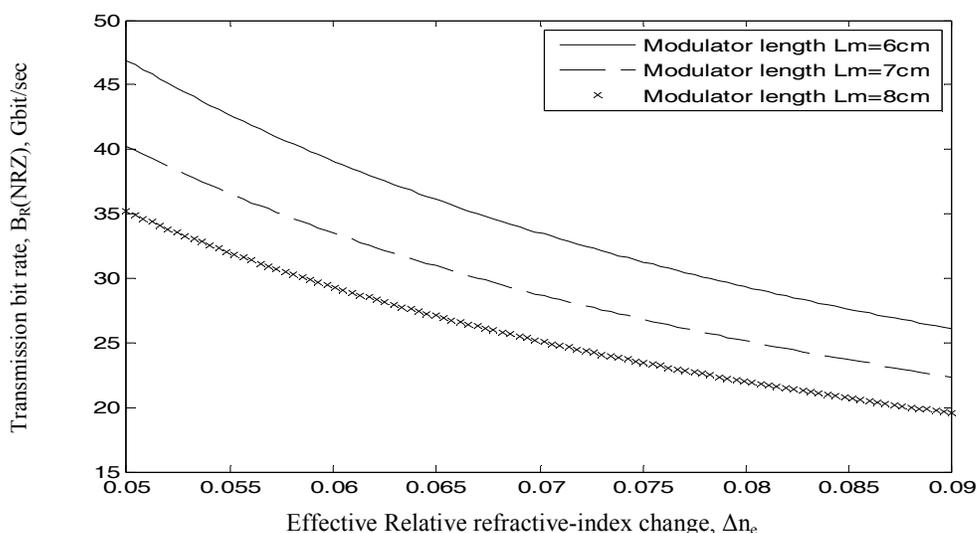
Fig. 12. Variations of transmission bit rate versus effective refractive index at the assumed set of parameters.
