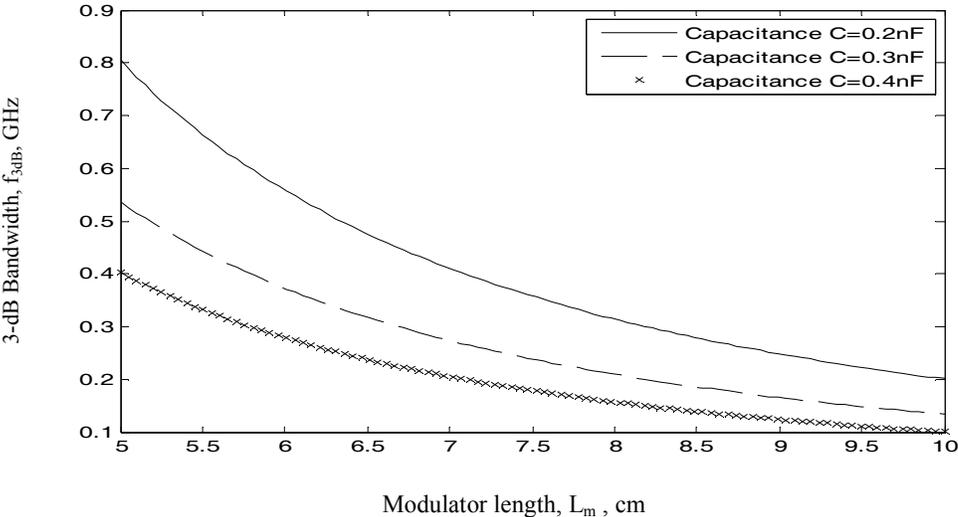
Fig. 10. Variations of 3-dB bandwidth against modulator length at the assumed set of parameters.
