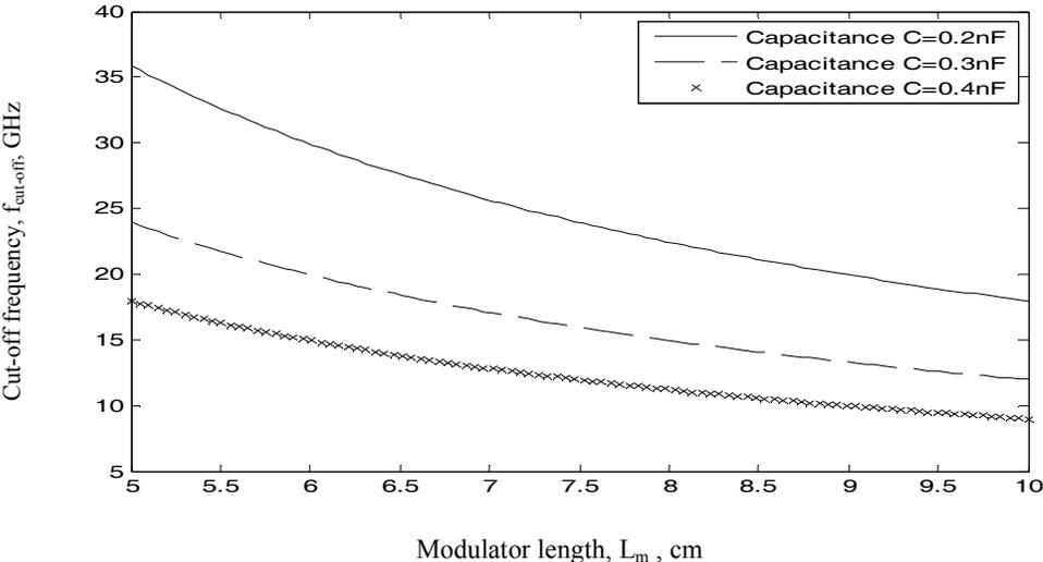
Fig. 8. Variations of cut-off frequency against modulator length at the assumed set of parameters.
