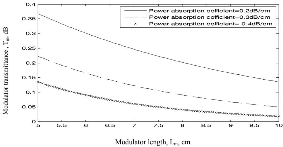
Fig. 6. Variations of the modulator transmittance against modulator length at the assumed set of parameters.
