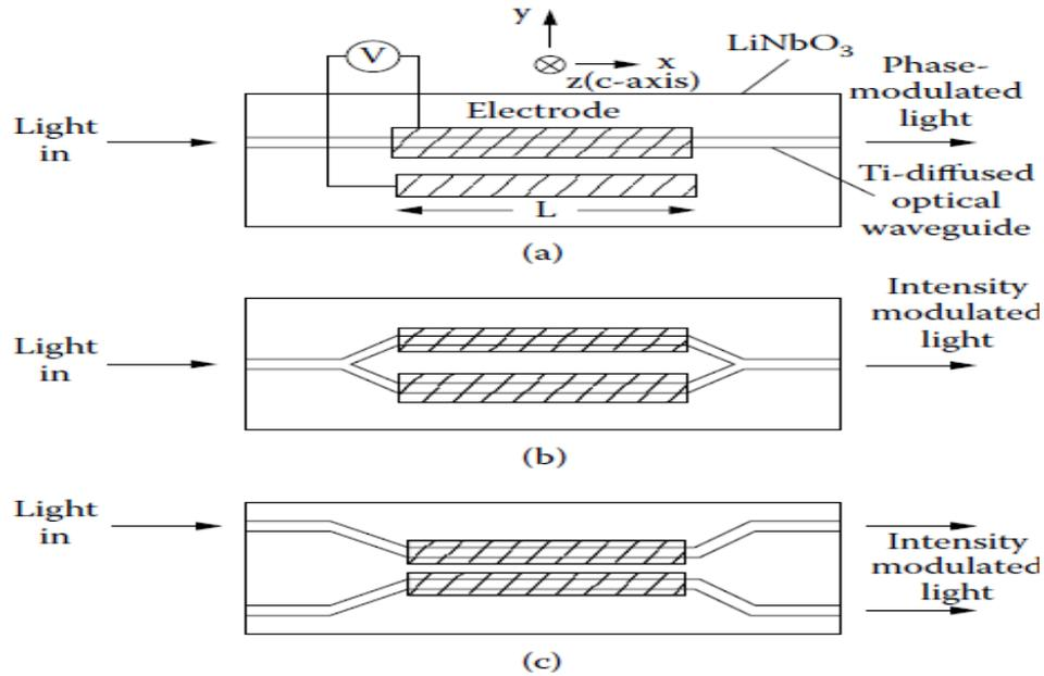
Fig. 1. Scheme of typical waveguided z-cut LiNbO<sub>3</sub> devices. (a) phase modulator, (b) intensity modulator using Mach-Zehnder interferometer, and (c) intensity modulator using directional coupler.
