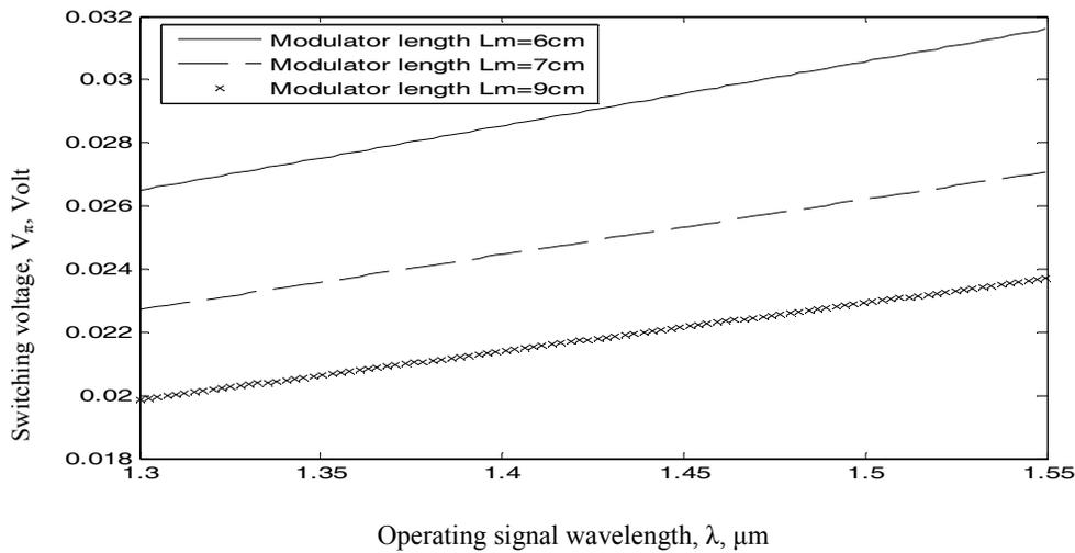
Fig. 3. Variations of the switching voltage versus operating signal wavelength at the assumed set of parameters.
