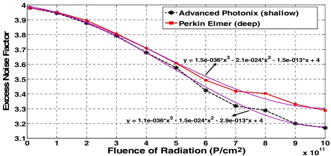
Fig. 4. Variations of the excess noise factor against fluence of radiation at the assumed set of parameters.
