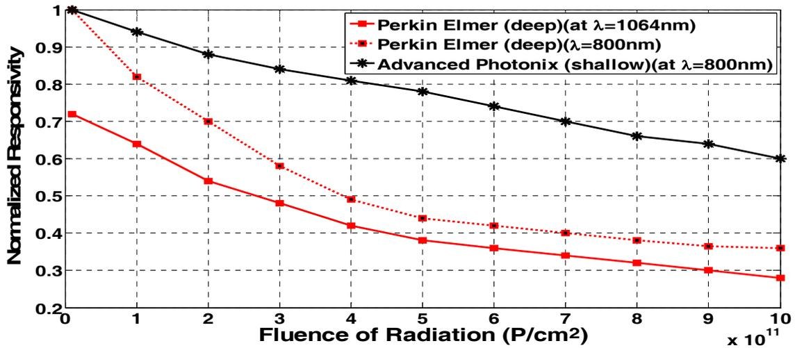
Fig. 7. Variations of the normalized responsivity against fluence of radiation at the assumed set of parameters.
