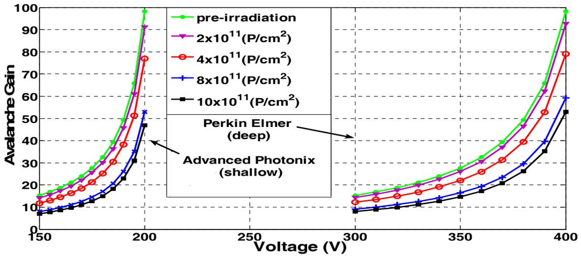
Fig. 6. Variations of the avalanche device gain against applied voltage at the assumed set of parameters.
