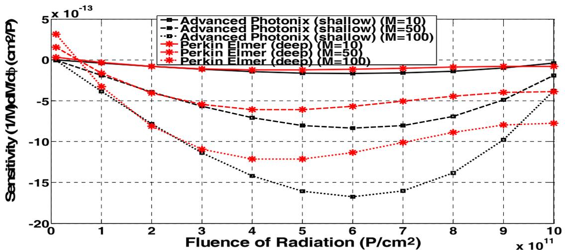
Fig. 11. Variations of the device irradiation sensitivity against fluence of radiation at the assumed set of parameters.
