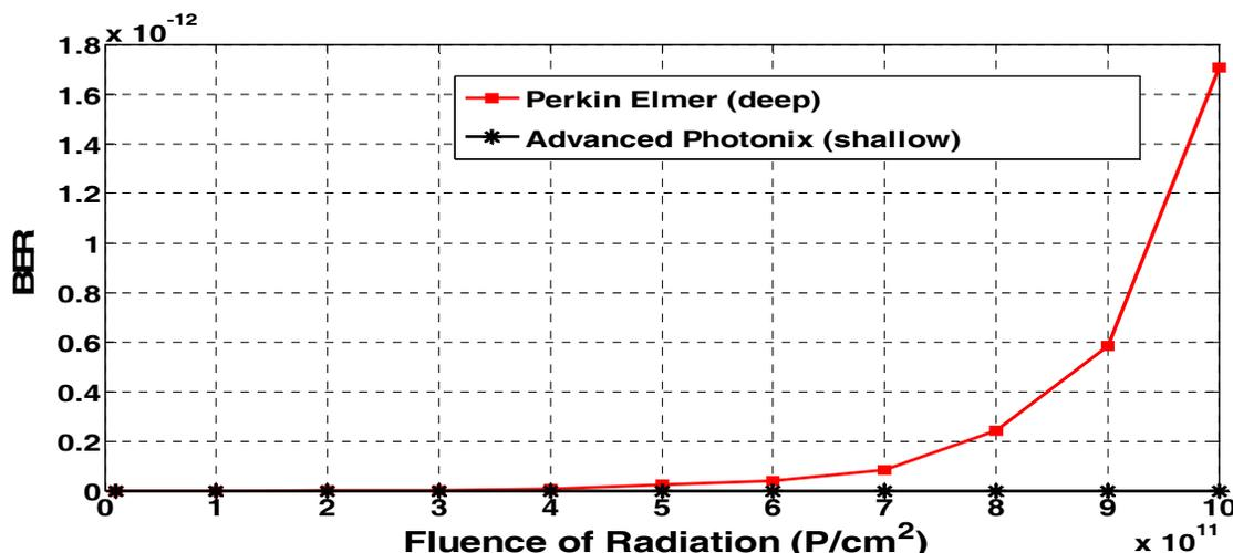
Fig. 12. Variations of the device irradiation BER against fluence of radiation at the assumed set of parameters.
