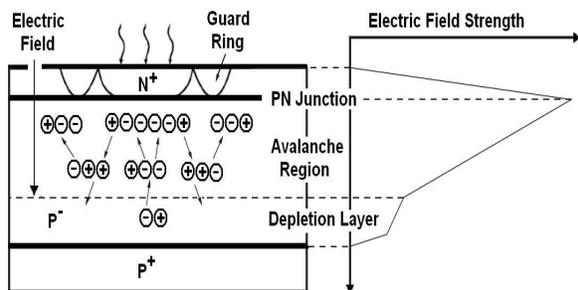
Fig. 1. Schematic of the avalanche process in an APD.
