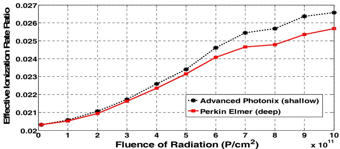
Fig. 5. Variations of the effective ionization rate ratio against fluence of radiation at the assumed set of parameters.
