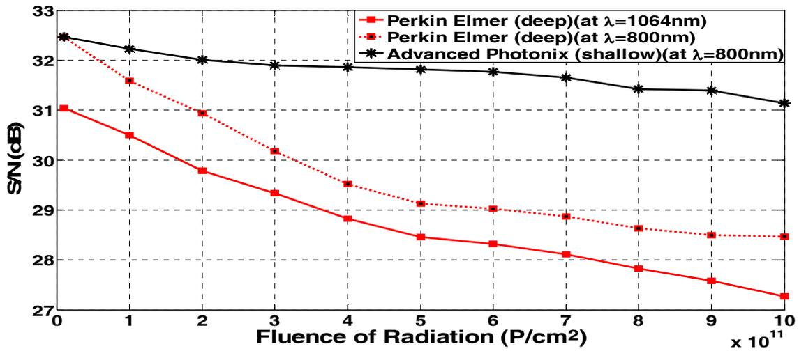
Fig. 9. Variations of the signal to noise ratio against fluence of radiation at the assumed set of parameters.
