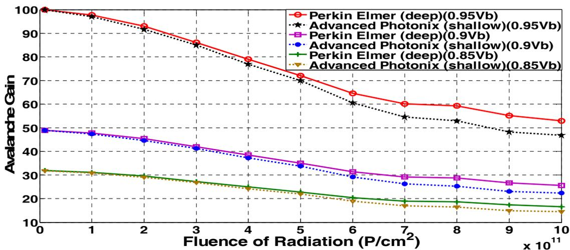
Fig. 2. Variations of avalanche gain against fluence of radiation at the assumed set of parameters.
