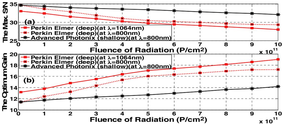
Fig. 10. Variations of both maximum signal to noise ratio and optimum gain against fluence of radiation at the assumed set of parameters.
