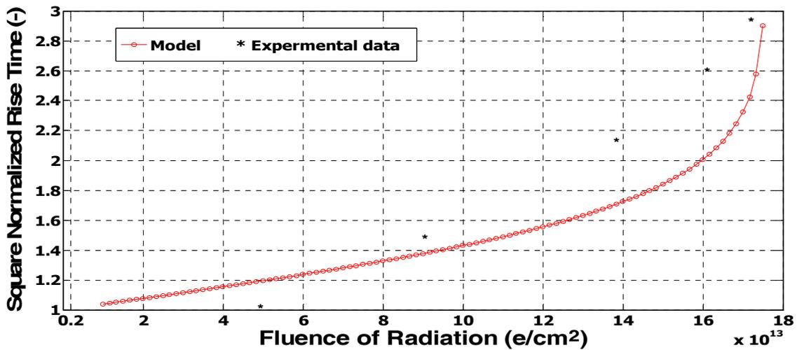
Fig. 8. Variations of the square normalized rise time against fluence of radiation at the assumed set of parameters.
