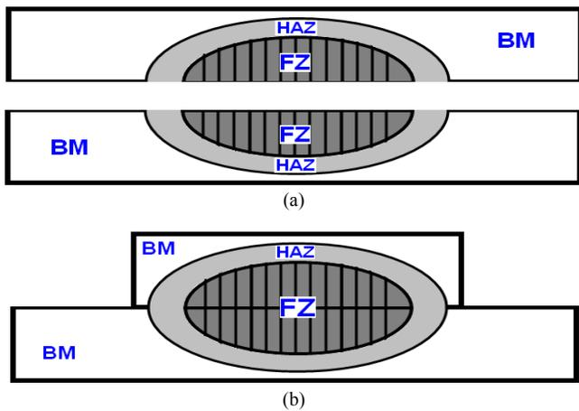
Fig.1: Schematic representation of main failure modes of spot welds: (a) interfacial and (b) pull-out
