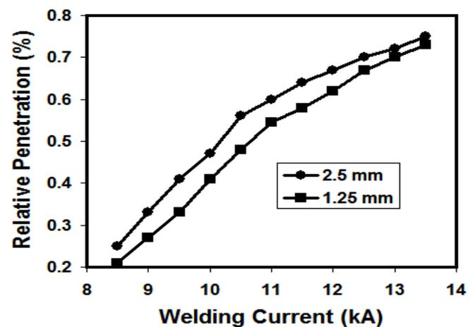
Fig. 5: Effect of welding current on the weld penetration
