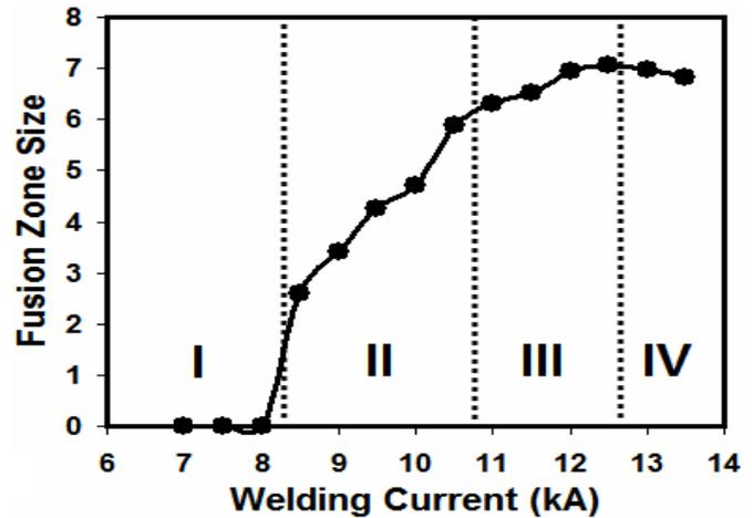
Fig. 4: Effect of welding current on the FZ size
