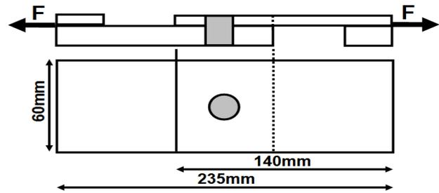
Fig. 2: Tensile-shear specimen dimensions
