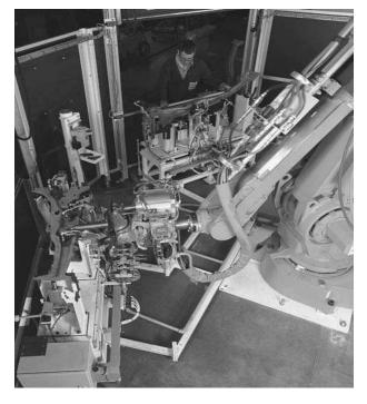
Fig. 3. Modern robotic resistance spot welding cell. The robot welds on one jig while the operator unloads/loads the second jig. Courtesy of British Federal
