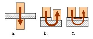
Fig. 8: Examples of resistance welding electrode configurations: a) direct, b) step, and c) series
