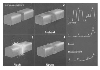
Fig. 6: Principles of flash butt welding. Courtesy of TWI Ltd
