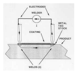
Fig.1: Principles of spot welding process
