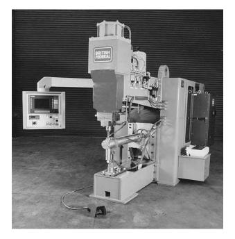
Fig. 2: Modern pedestal mounted spot welder for aerospace applications
