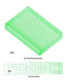
Fig. 4: Finite-Element Modeling of Resistance Welding
