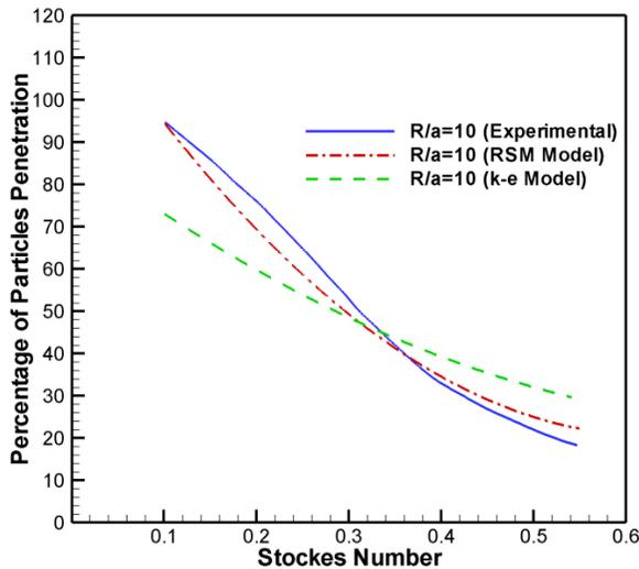
Fig. 5. K-epsilon Model in comparison with RSM and experimental samples
