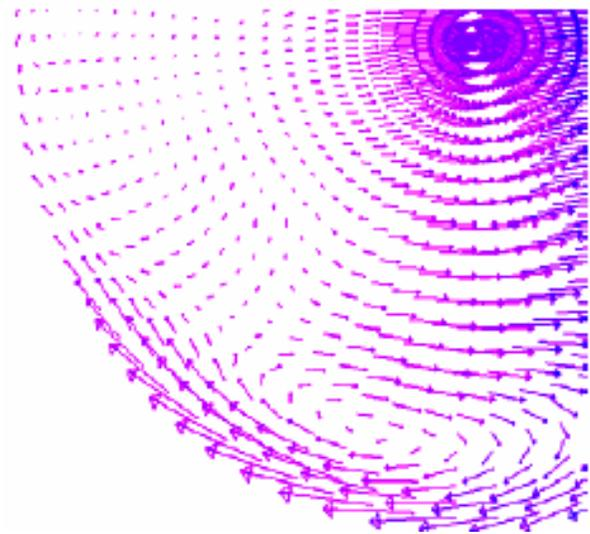
Fig. 3. Velocity vectors in downstream of bend exit plane
