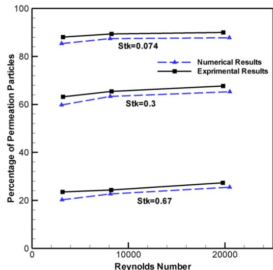
Fig. 7. Percentage of particles penetration versus Reynolds number
