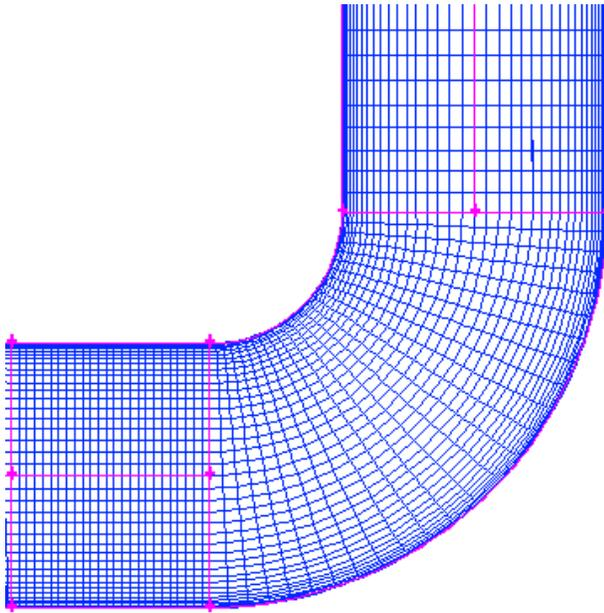
Fig. 2. The manner of grid generation at pipe- knee junction
