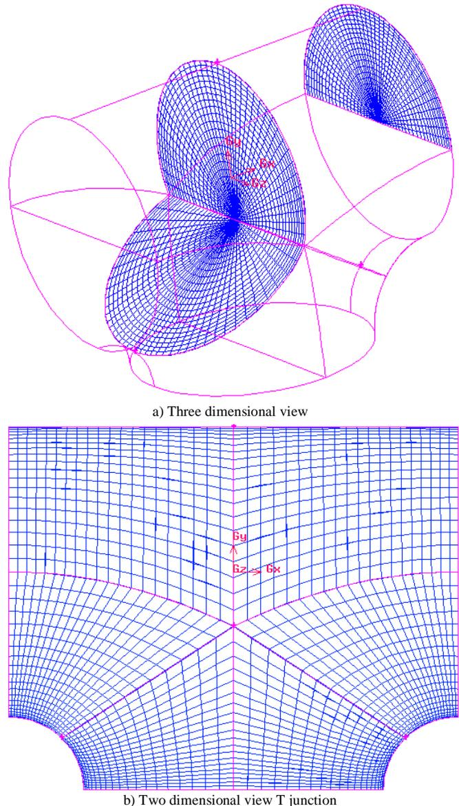
Fig. 1. The manner of grid generation at three way
