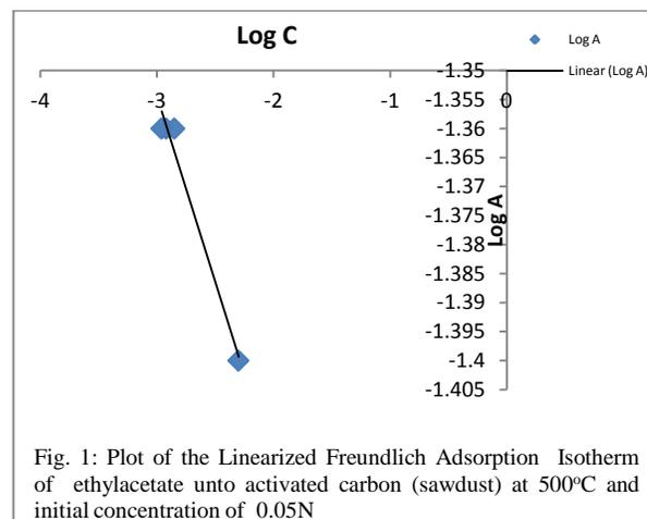
Fig. 1: Plot of the Linearized Freundlich Adsorption Isotherm of ethylacetate unto activated carbon (sawdust) at 500°C and initial concentration of 0.05N
