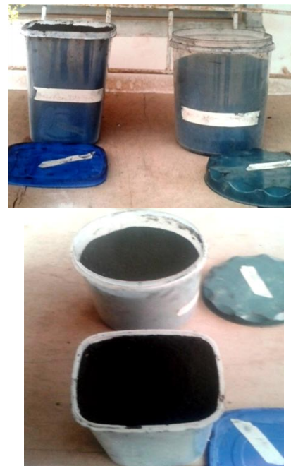
Fig. 8: Samples of Carbon Black collected from filters, conical section
