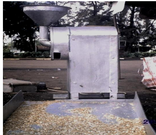
Fig. 11: Photograph of Melon Dehusking Machine by Principle of Impact
