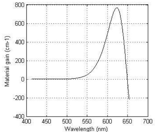
Fig. 2. Plot of material gain vs. wave length with the maximum gain  $770cm^{-1}$  at around 625nm wave length
