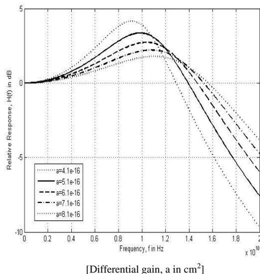
Fig. 9. Plots of relative response vs. frequency of  $\text{Ga}_{0.5}\text{In}_{0.5}\text{P}/(\text{Al}_{0.5}\text{Ga}_{0.5})_{0.5}\text{In}_{0.5}\text{P}$  at 300K with the variation of differential gain at injection current 90mA
