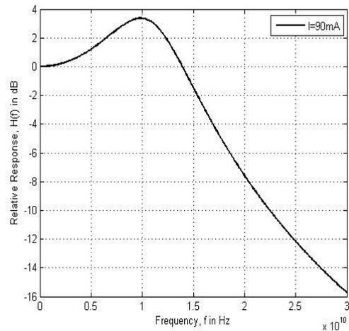
Fig. 7. Plot of relative response vs. Frequency of  $\text{Ga}_{0.5}\text{In}_{0.5}\text{P}/(\text{Al}_{0.7}\text{Ga}_{0.3})_{0.5}\text{In}_{0.5}\text{P}$  at 300K
