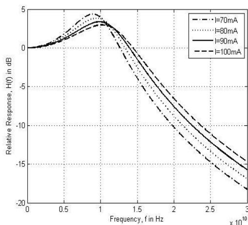
Fig. 8. Plots of relative response vs. frequency of  $\text{Ga}_{0.5}\text{In}_{0.5}\text{P}/(\text{Al}_{0.5}\text{Ga}_{0.5})_{0.5}\text{In}_{0.5}\text{P}$  at 300K with the variation of injection current
