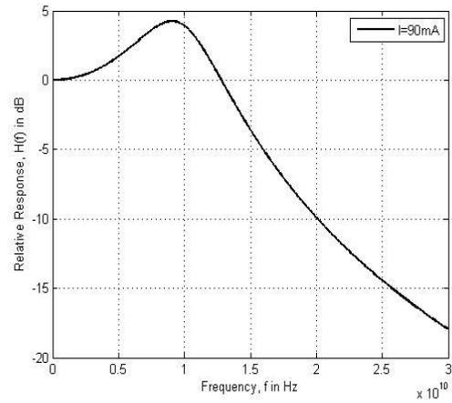
Fig. 11. Plot of relative response vs. Frequency of  $Ga_{0.5}In_{0.5}P/(Al_{0.7}Ga_{0.3})_{0.5}In_{0.5}P$  at 300K with the variation of width of active region ( $8 \times 10^{-4}$  cm). The resonance frequency is obtained 8 GHz and the modulation bandwidth around 14 GHz at 90mA
