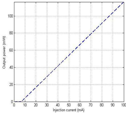
Fig. 4. Plot of Output power vs. Injection current of the designed red laser at 300K maintaining injection current 90mA
