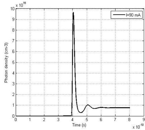
Fig. 6. Plot of Photon density vs. Time. The steady state photon density at 90 mA is found  $8.763 \times 10^{15} \text{ cm}^{-3}$
