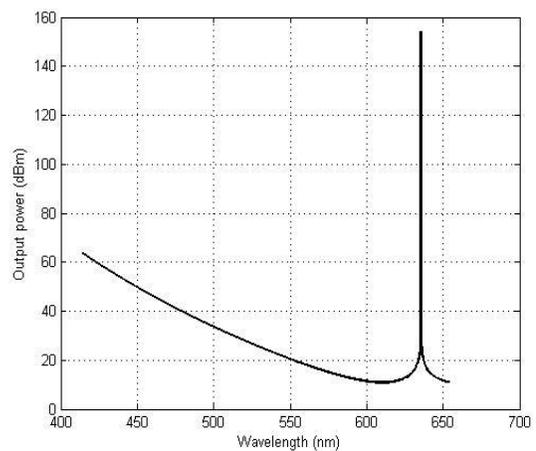
Fig. 3. Plot of power vs. wavelength of the designed red laser at 300K. A peak intensity of the power is obtained at 635nm wavelength
