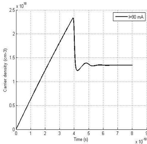
Fig. 5. Plot of Carrier density vs. Time. The steady state carrier density of  $1.365 \times 10^{18} \text{ cm}^{-3}$  is found at 90mA
