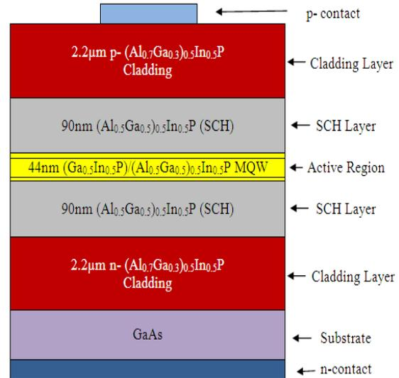
Fig. 1. Structure of designed 635nm MQW Red Laser
