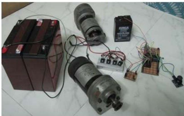
Fig. 4: Electro-mechanical structure parts consisting of Batteries, Motors, Joystick and Circuit Board
