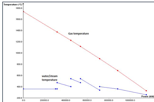
Fig. 4: Temperature-heat (T-Q) diagram of boiler (without air heater) at 100 % load
