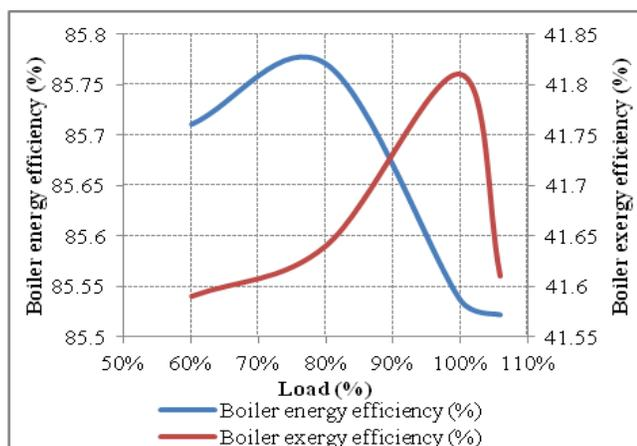
Fig. 3: Boiler energy and exergy efficiency
