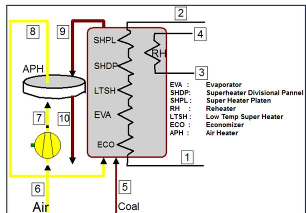
Fig. 2: Display of thermodynamic state of boiler model with arrangement
