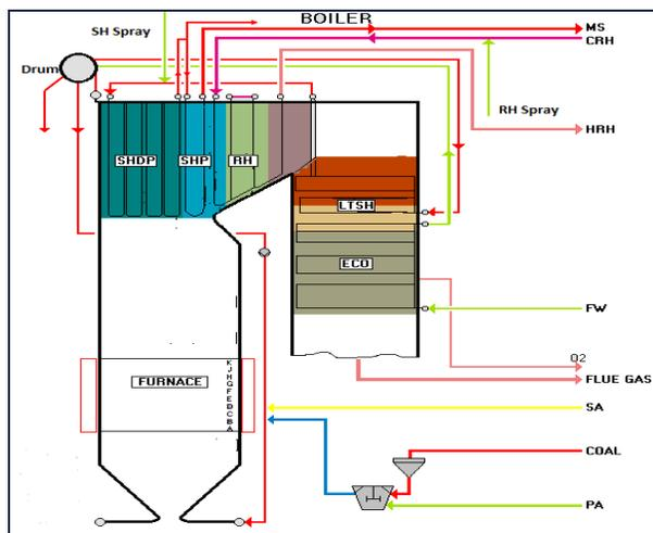
Fig. 1: Schematic diagram of boiler
