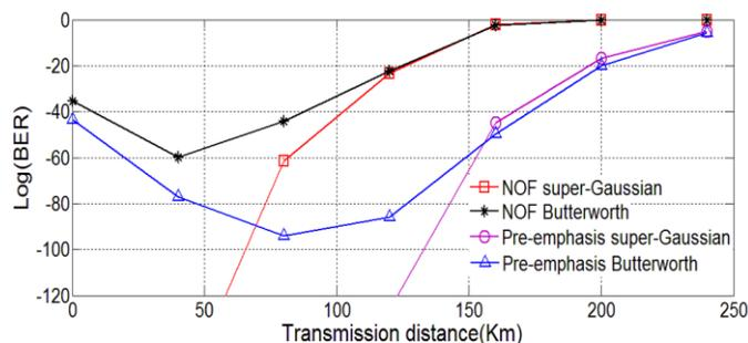
Fig.7. BER and transmission distance relationship for NOF and pre-emphasis techniques.
