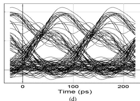
Fig. 8. Eye patterns at 150 km of SMF. (a) pre-emphasis with super-Gaussian filter, (b) pre-emphasis with Butterworth filter, (c) NOF with super-Gaussian filter and (d) NOF with Butterworth filter
