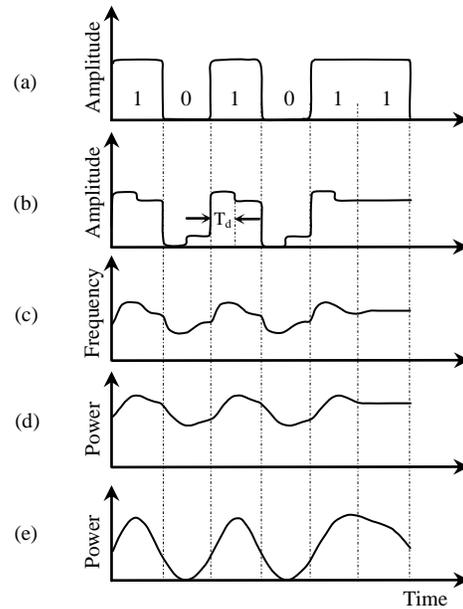
Fig. 3. Operation principle of transmitter. (a) NRZ signal, (b) pre-emphasis signal to drive VCSEL, (c) frequency profile (Chirp) of VCSEL, (d) optical power at the VCSEL output and (e) OBPF output power
