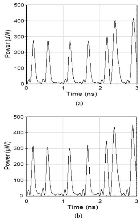
Fig. 4. Receiver input power without pre-emphasis. (a) super-Gaussian filter and (b) Butterworth filter for 010001000001000010000101100011 bit sequence
