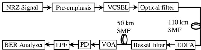
Fig. 2. VCSEL based transmitter with pre-emphasis and filtering scheme in optical transmission system
