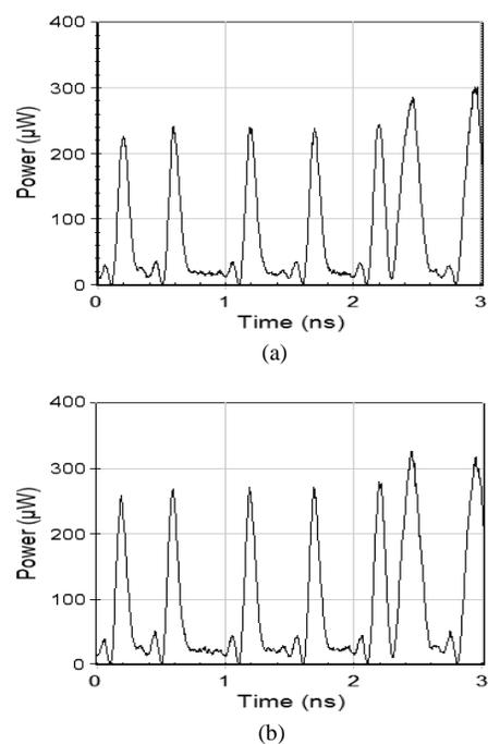
Fig. 5. Receiver input power with pre-emphasis. (a) super-Gaussian filter and (b) Butterworth filter for 010001000001000010000101100011 bit sequence
