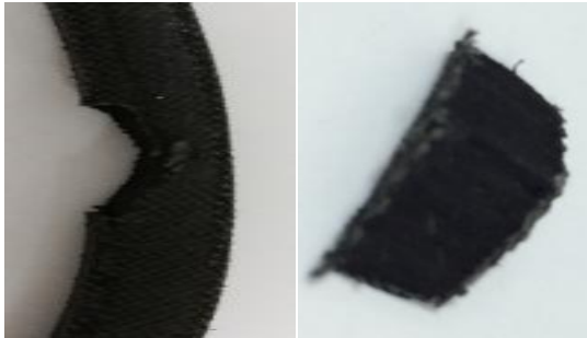
Fig. 19. Loose and Side Cut and removed piece
