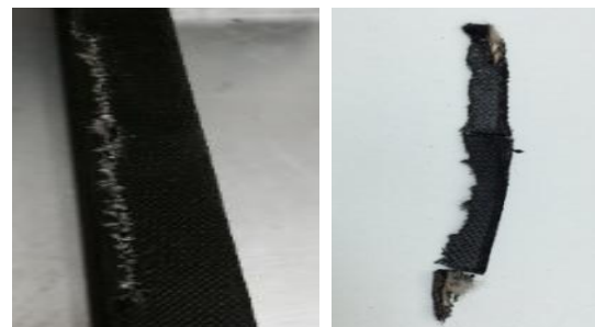
Fig. 18. Side Cut and removed piece
