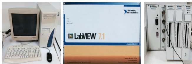
Fig. 15. LabVIEW® software integrated with DAQ module
