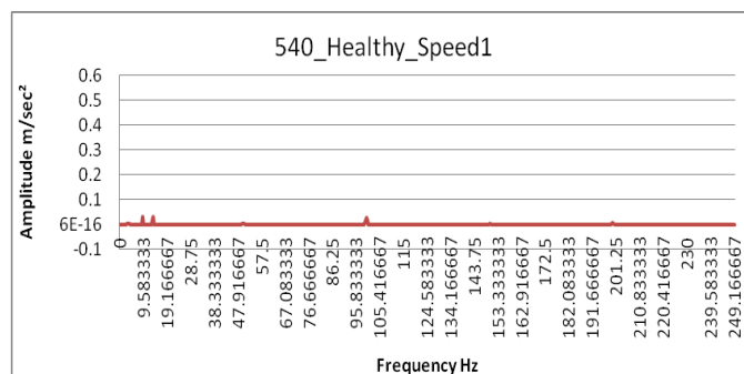
Fig. 21. Acceleration with frequency at speed of 540 rpm
