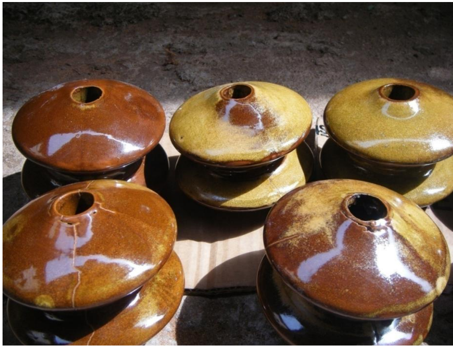
Plate 4: Glazed and gloss fired electrical porcelain insulator
