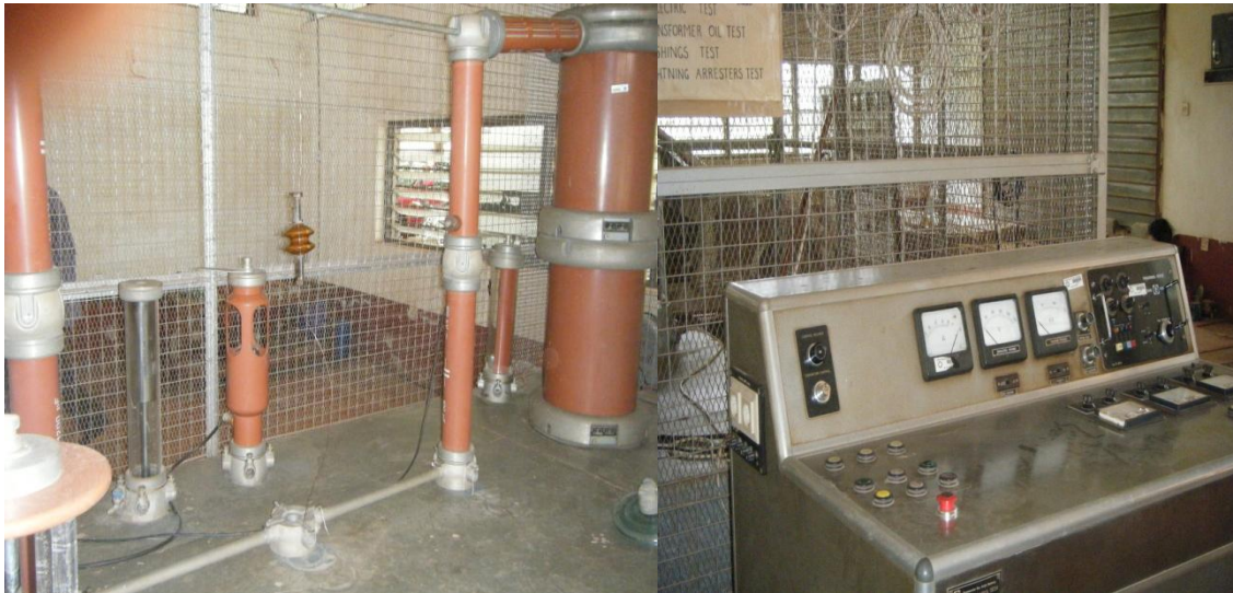
Plate 2. Experimental set-up for breakdown voltage test
