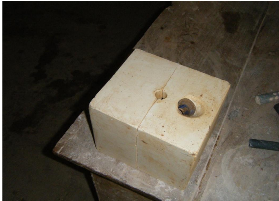
Plate 1: POP Mould for shackle insulators used for the study
