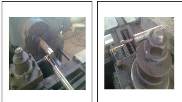
Fig. 2. Dry orthogonal turning of mild steel sample and cutting force measurement on tool using dynamometer [7]
