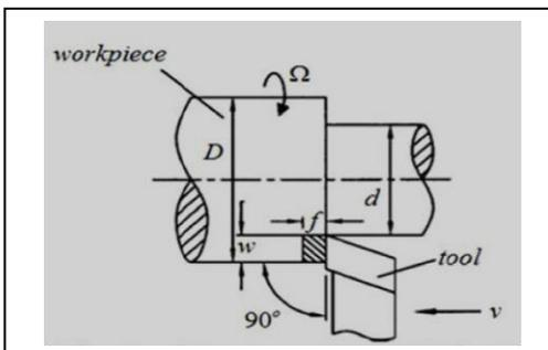
Fig. 1. Orthogonal turning with cutting parameters [1]
