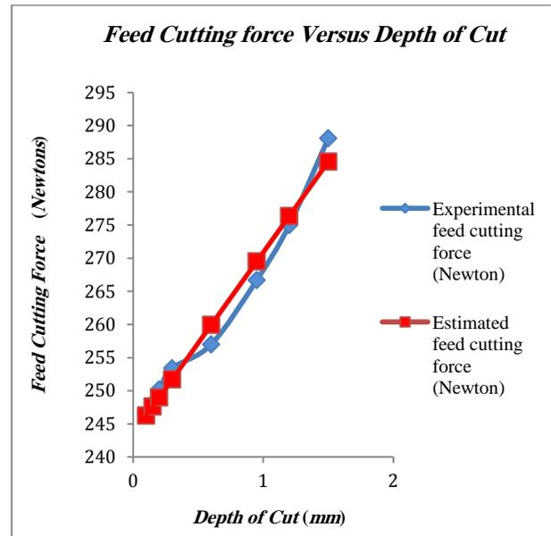
Fig. 3. Feed cutting force versus depth of cut
