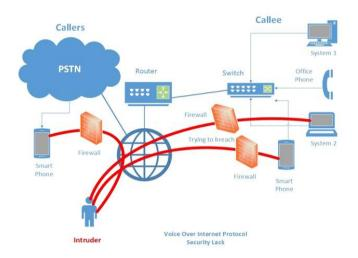
Fig. 2: VoIP Security with firewall
